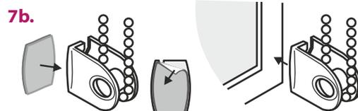
7. Install the cord tension device on the wall (Drawing 7a) or directly onto the window frame with double sided tape (Drawing 7b), in a position that will keep the cord taut and secure. Please note screws are not included in the pack
