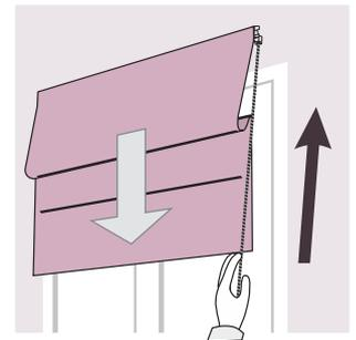
After releasing the locking system, release the cord to fully close the blind.
