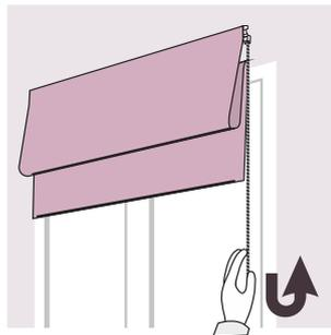
Slowly and gently release the cord at a required height to lock the blind in this position.
