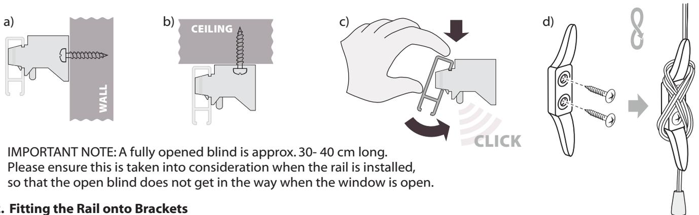
**IMPORTANT NOTE:** A fully opened blind is approx. 30- 40 cm long. Please ensure this is taken into consideration when the rail is installed, so that the open blind does not get in the way when the window is open.
